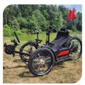
We specialise in the design of customised comfort, expedition and rehabilitation bicycles. The innovative designs combine the features of a recumbent bicycle with the potential of off-road vehicles. Thanks to the technologies used, the bikes are not only very comfortable, but also provide a sense of stability when riding, even under heavy loads.
